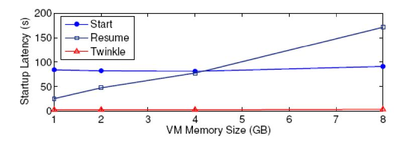
Startup latency of RUBiS service within JBoss which runs on Dell PowerEdge blade servers with Intel 5620 CPU, 24 GB RAM and 10K RPM SAS disks.
