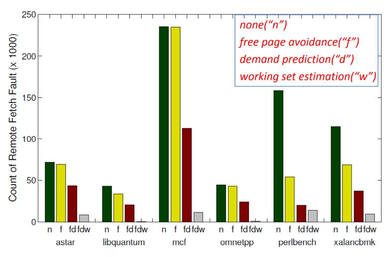
The count of remote page faults under different combinations of techniques.
