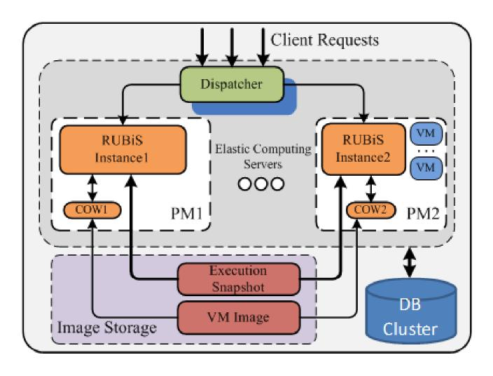
Example of a cloud data center employing fast restart mechanism.
