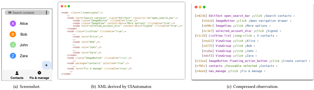
Figure 8: An example of the screenshot, original XML and compressed observation of Contacts APP page.
