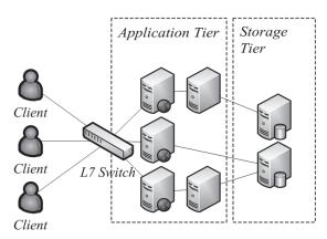
Figure 5. Architecture of a Web application
