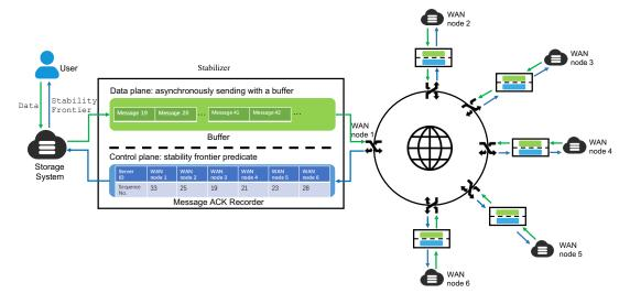
Fig. 1. Stabilizer system overview: structure, workflow, data plane, and control plane
