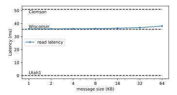
Fig. 3. Latency of read operation
